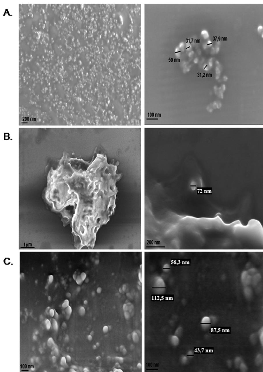
**Fig. 2.** Scanning electron microscopy micrographs of the powder particles, dispersed in acetone, based on a crude extract of carotenoids of the Cantaloupe melon pulp (*Cucumis melo* L. *reticulatus* Naud.) and encapsulating agents obtained by emulsification O/W technique. (A) EPG: encapsulated in porcine gelatin, (B) EWPI: encapsulated in whey protein isolate and, (C) EWPC: encapsulated in whey protein concentrate.
