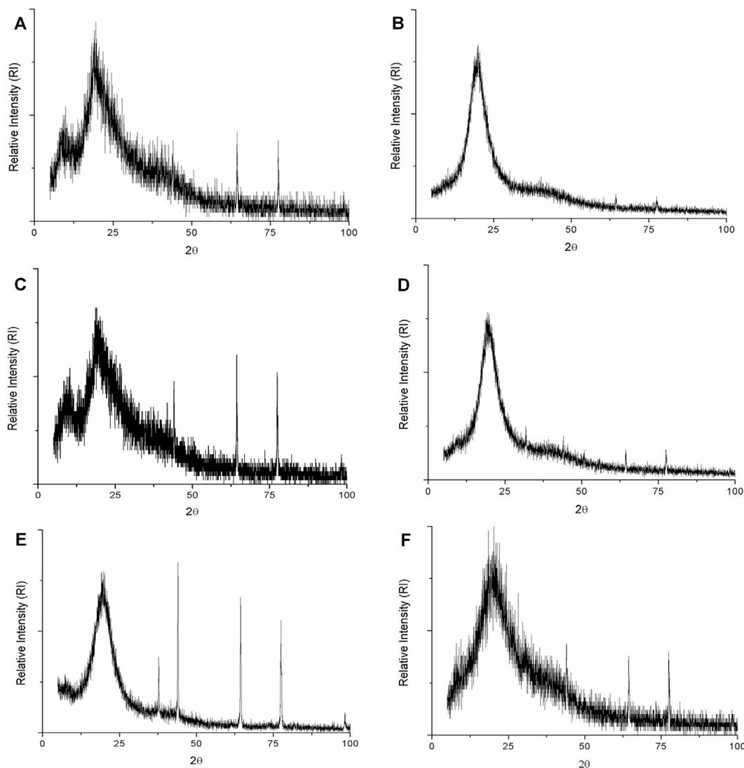
**Fig. 4.** X-ray diffraction of the powder particles based on a crude extract of carotenoids of the Cantaloupe melon pulp (*Cucumis melo* L. *reticulatus* Naud.) and encapsulating agents obtained by emulsification O/W technique. (A) WPC: whey protein concentrate; (B) EWPC: encapsulated in whey protein concentrate; (C) WPI: whey protein isolate; (D) EWPI: encapsulated in whey protein isolate; (E) PG: porcine gelatin; and (F) EPG: encapsulated in porcine gelatin.
